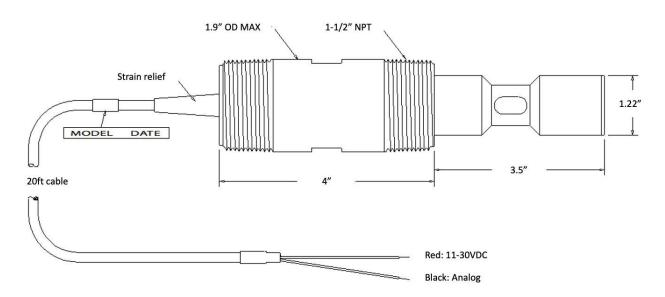
4-20 mA output, CPVC body with 1.5" MNPT thread fitting
