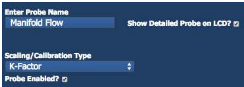
Figure 6-15 - The only choice for Scaling Type/Calibration for a pulse input probe is K-Factor.
