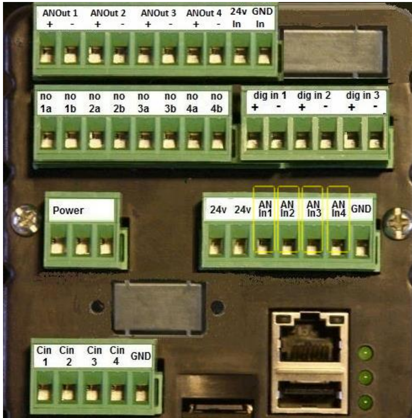
Figure 7-4 - During set-up of an analog probe to a 2300 with an analog output card, the analog output connector (on top) appears.
