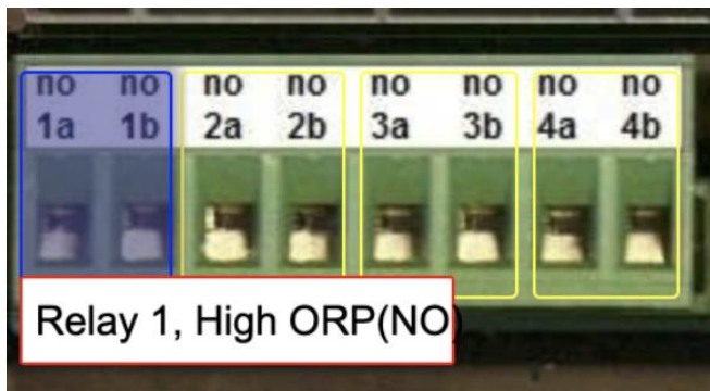
Figure 6-12 - Relay connections on the back of the 2300. The yellow rectangles show relays that are unused. The shaded blue rectangle over Relay 1 shows a relay that is configured for a previous sensor and a text box lists the relay function. You can still select that relay for another probe.
