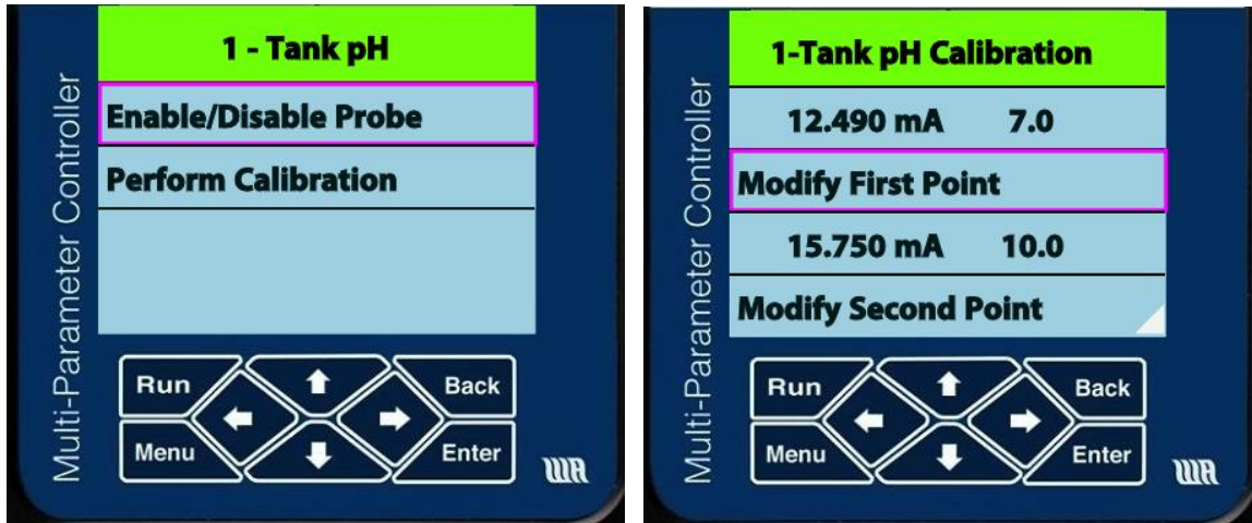
Figure 3-4 – Select Probe Calibration and then select 1 or 2 points at which to calibrate.
