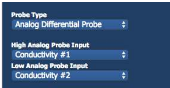
Figure 6-23 - Section of the Probe Selection page showing the definition of the differential sensor.
