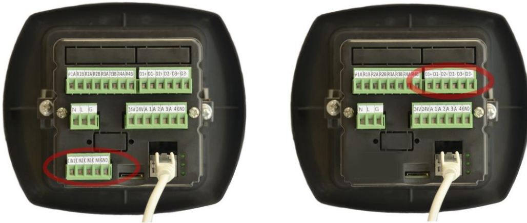
Figure 6-11 - The first 2300 version, shown on left, has two sets of contacts connecting a switch to reset the totalizer on a separate connector (C1-C4). The most recent version has no separate connector for a switch. However, any two connectors on the pulse (or "digital") connector can be used as an input for a switch.
