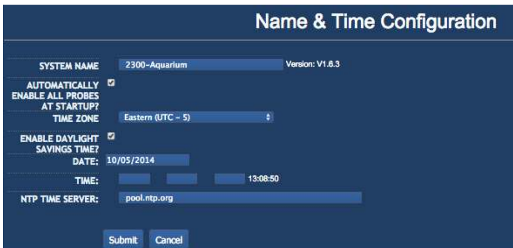
Figure 5-12 - Name & Time Configuration allows you to set the 2300 name and time of day.
