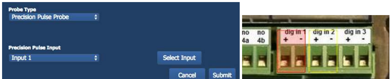
Figure 6-14 – The New Probe Wizard screen allows the user to choose either of the two Precision Pulse Inputs or the single Pulse input . The right hand photo shows the red rectangle.
