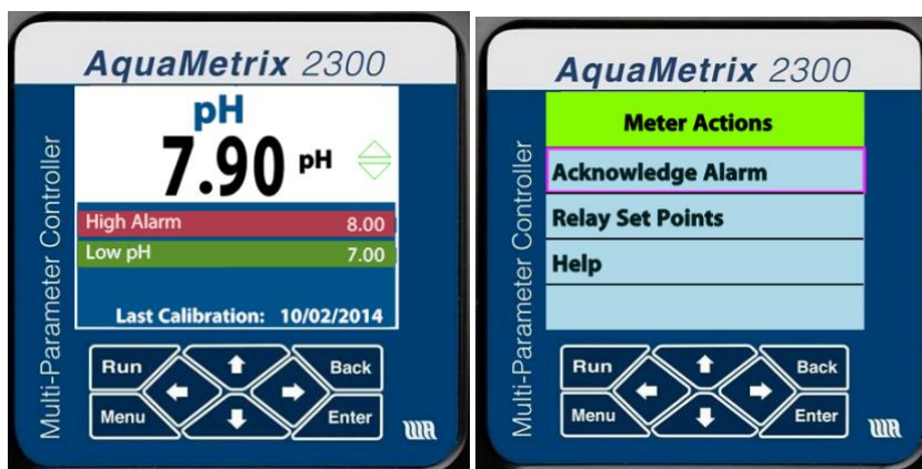
Figure 6-10 - The bar around the High Alarm alert flashes red until you press the Enter button. Pressing the Enter button on the Meter Actions screen brings you back to the screen on the left—only this time with a steady red bar.
