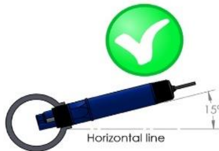
Horizontal or upside down installations are not acceptable
